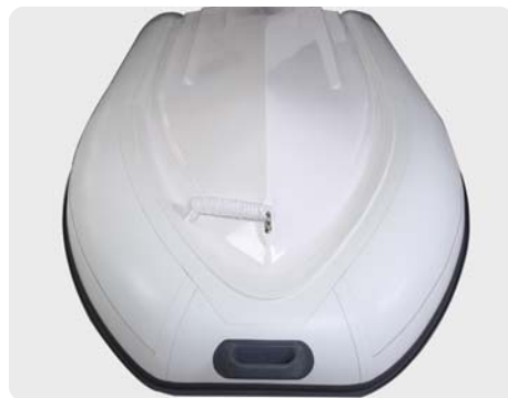
V-shaped polyester hull features two ridges for increased stability and safe turns.
