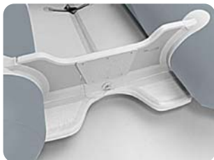
V-shape rigid inflatable hull (Pi230VB, Pi270VB & Pi320VB).
