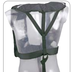
Y-shaped 25 mm polypropylene straps hold the lifejacket flat on the back and prevent air trapped in the jacket. Also contribute to a better weight distribution on the shoulders.
