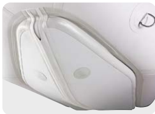
V-shape rigid inflatable hull (Pi230VB, Pi270VB & Pi320VB).
