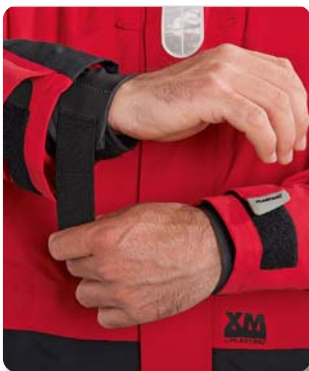
Adjustable double cuffs : outer cuff adjusts with elasticated tightening tab ; inner cuff waterproofness is ensured by a PU seal.
